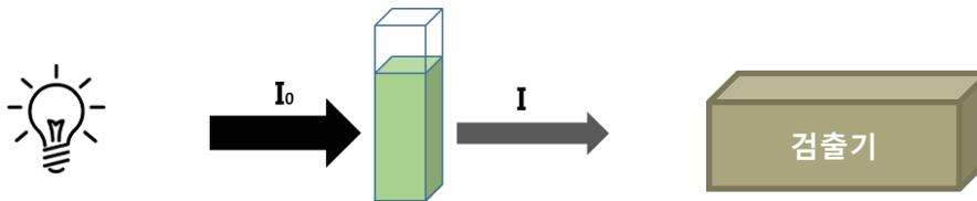
Transmittancy: the ratio of transmitted radiation to the incident radiation; it is expressed in the following equation.
